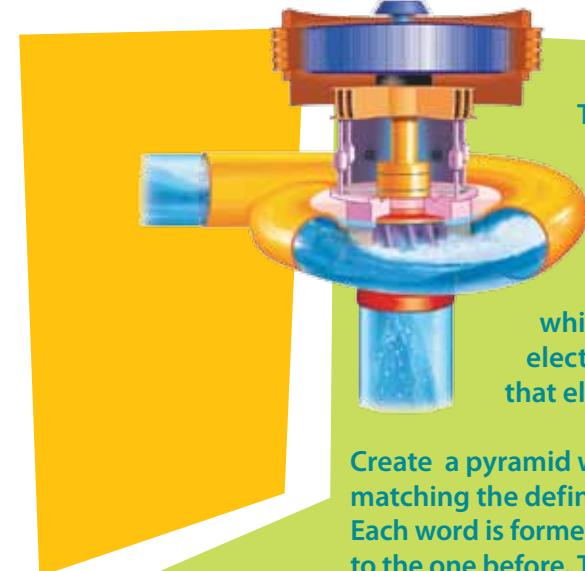
The mechanical energy of water flowing through a turbine is transmitted to the generator, which converts it into electricity. What brings that electricity to users?
