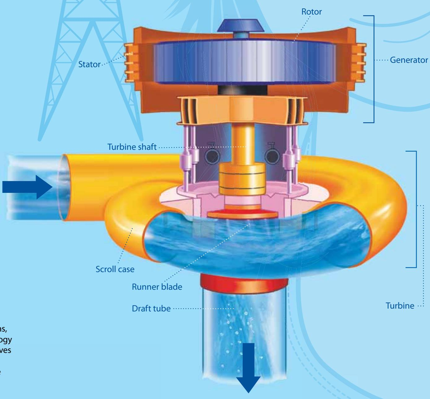
When there isn't enough of a drop in level to give water the necessary driving force, the turbine is installed underground.
