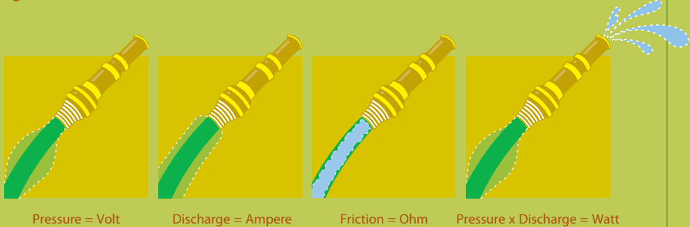
Figure 1 – Similarities between the water in a hose and an electric current
