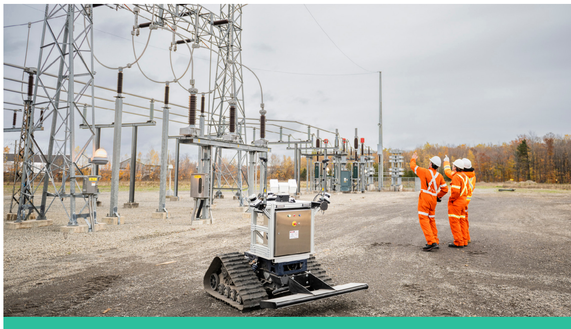
Designed to inspect transmission substations, the robotic vehicle known as RIAUEP is one of our many technological solutions. The robot was featured in the December 2022 edition of HydroPresse .
